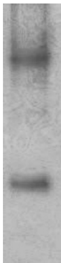
Figure 1. SDS-PAGE (12.6% gel) of Dominga grape PPO stained with 5 mM L-DOPA and 3 mM MBTH in 10 mM sodium acetate buffer (pH 3.0).
